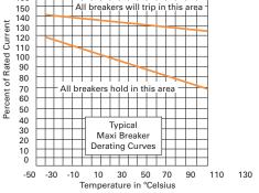
These curves are to be used only as a guide in selecting a protector for a particular application. Factors such as distance from the heat source and the method of mounting should be considered in selecting a protector. Final trip times are dependent upon terminal configuration and mounting in the application.
